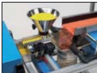
HAVER-CPA: Photo-optical particle analysis for a measuring range from 0,025 mm up to 400 mm
